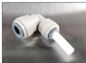
To prevent damage to the seals: Always use a wrench or a screwdriver to push back the grey release ring if the hose must be removed or replaced.
