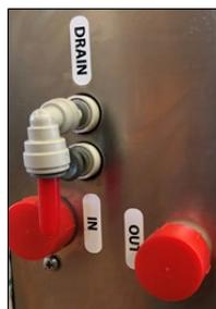
Connect the drain hose. Push the grey release ring back with a screwdriver or a wrench and remove the red plastic plug from the elbow. If you pull out the plug without pushing the release ring, this will damage the seal. Press the 8 mm drain hose firmly into the knee and put the outlet side of the tube into the sewer drain.
